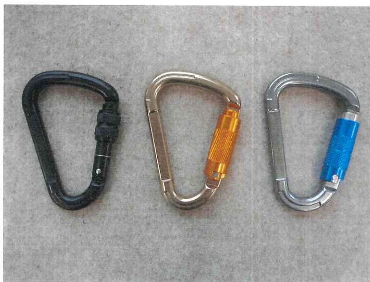
Carabiner, type A713KSG (screw), der. var. A713KTL (twist lock) / A713KTL-3 (triple lock)
